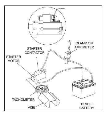
Figure 17. Testing Starter Motor Performance
